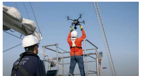
A pilot on deck operates the drone whilst a catcher launches and retrieves the drone.
