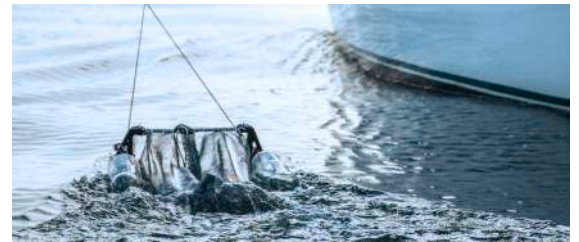
A special net, dragged along the side of the Sea Ranger vessel, collecting microplastics at the water surface.
